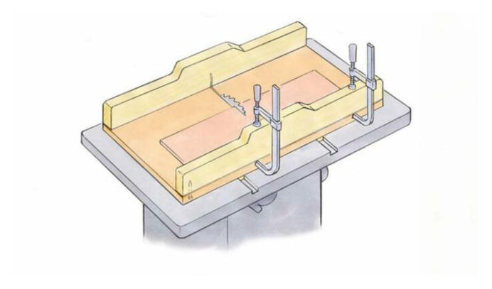
Most of us end up building a number of table-saw sleds over the years. The toughest part is lining up the main fence so it's perfectly square with the blade.
